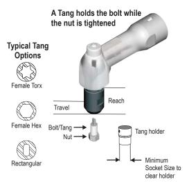
**NOTE:** The bolt can extend beyond the nut no more than the specified Travel distance when tightened.
