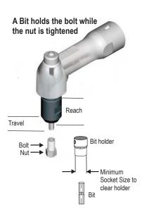
**NOTE:** The bolt can extend beyond the nut no more than the specified Travel distance when tightened.
