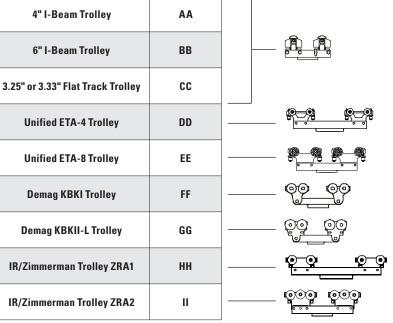
**Note:** Single Trolleys not recommended for torque reaction applications.
