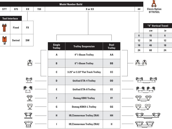
Note: Single Trolleys not recommended for torque reaction applications.
