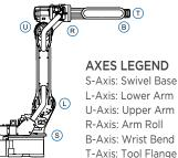
AXES LEGEND S-Axis: Swivel Base L-Axis: Lower Arm U-Axis: Upper Arm R-Axis: Arm Roll B-Axis: Wrist Bend
